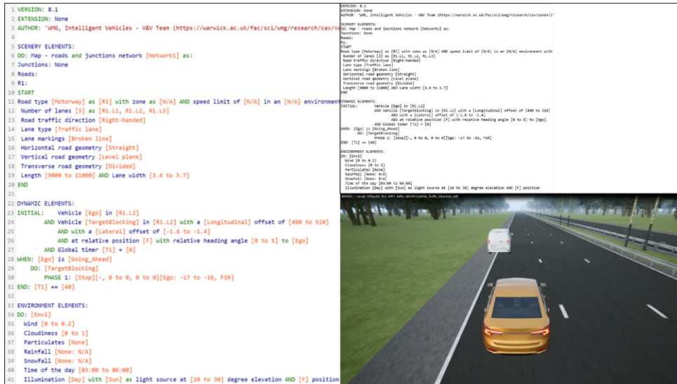
Figure 19: Example SafetyPool™ Scenario database dynamic scenario in Scenario Description Language level 2, level 1 and visualisation (please note SDL 1 and 2 are right hand drive scenarios, and the visualisation has been converted to represent left hand drive through the relevant toolchain).
